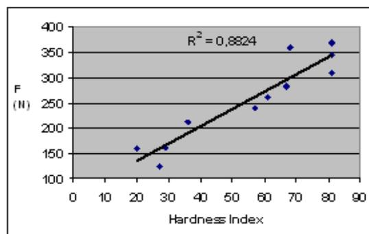
**Fig. 3.** Connection between the breaking force (F) and the Hardness Index (set “B”, vertical position, moisture content: 13.52%)
