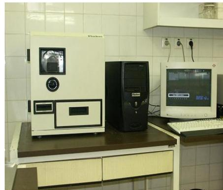
Fig. 2. Perten Single Kernel Characterization System (SKCS) 4100 device
