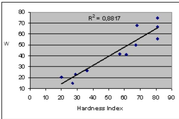
**Fig. 4.** Connection between the breaking work ( $W$ ) and the Hardness Index (set "B", vertical position, moisture content: 13.52%)
