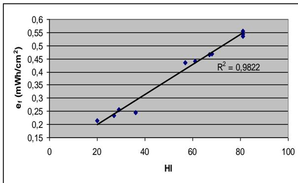
**Fig. 5.** Connection between specific grinding energy demand ( $e_g$ ) and the Hardness Index (set "B", moisture content: 13.52%)
