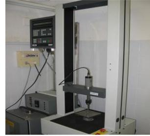
Fig. 1. Lloyd 1000R Testing Machines
