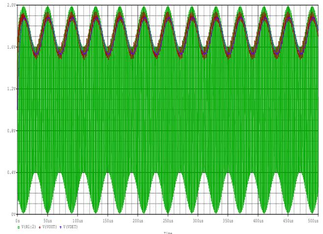
Fig.8 Peak detector operation in a time domain simulation
