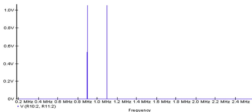
Fig. 6. The spectrum of the signal provided at the output of the multiplier (amplitude signal 20mV)
