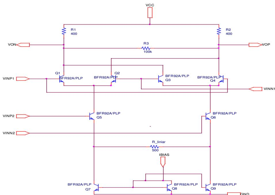
Fig.5. Multiplier circuit
