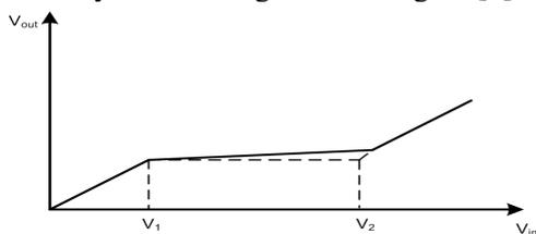
Fig. 2. The ideal transfer function of an AGC
