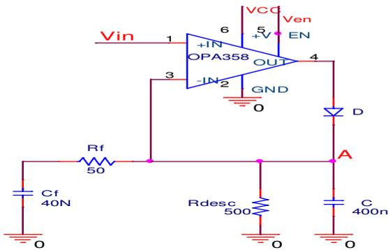
Fig.7. Peak detector circuit
