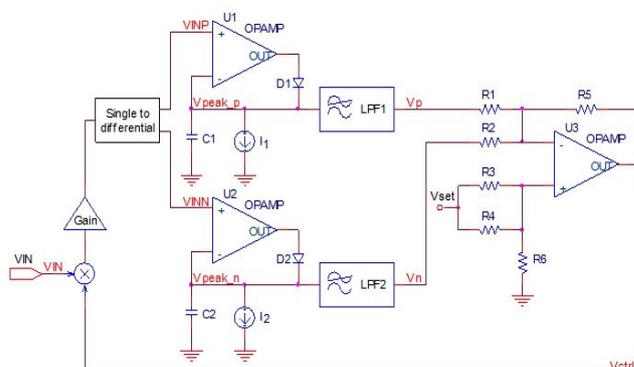
Fig. 3. AGC block diagram with feedback loop
