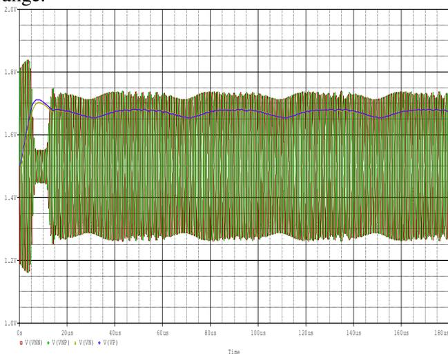
**Fig. 11.** The differential input signals (VNN, VPN) and the positive/negative envelopes
