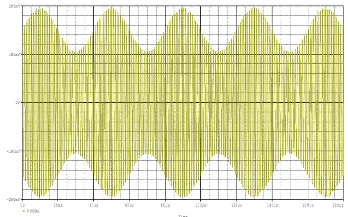
Fig.9. Amplitude Modulation test signal
