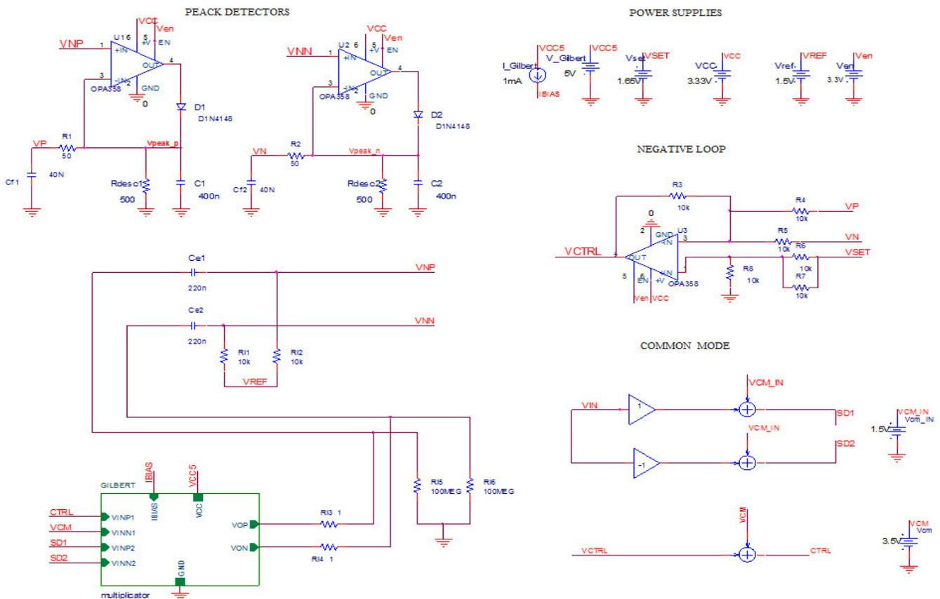
Fig. 4. AGC simulation circuit
