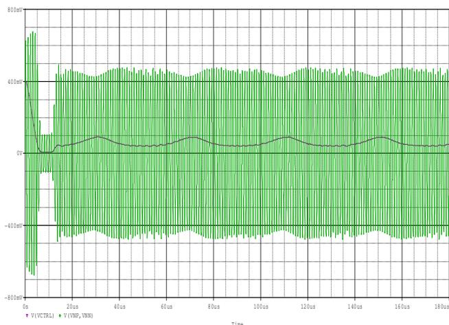
**Fig. 10.** The differential output signal (VNN, VPN) and the control signal ( $V_{ctrl}$ )
