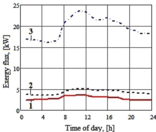
Fig.5. Variation of exergy of useful heat obtained in: 1 - HE, 2 - CHP for domestic hot water, 3 - CHP for district heating
