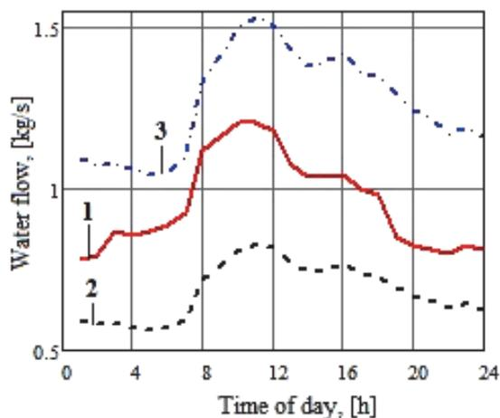
**Fig.3.** Variation of water flow obtained in: 1 - HE, 2 - CHP for domestic hot water, 3 - CHP for district
