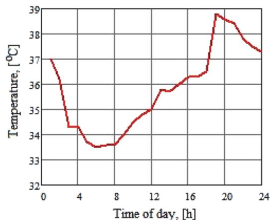
**Fig.2.** Variation of water temperature obtained from the heat exchanger
