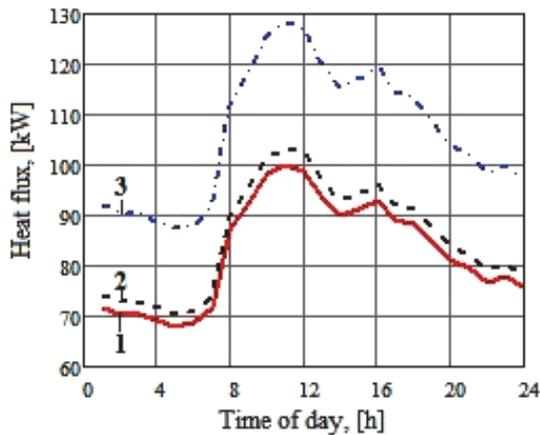
Fig.4. Variation of useful heat flux obtained in: 1 - HE, 2 - CHP for domestic hot water, 3 - CHP for district heating
