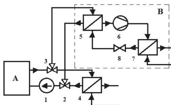
**Fig.1.** Heat recovery scheme: A-transformer; B-compression heat pump; 1-oil pump; 2, 3 - three-way valves; 4-oil-water heat exchanger; 5-evaporator; 6-compressor; 7-condenser; 8- expansion valve
