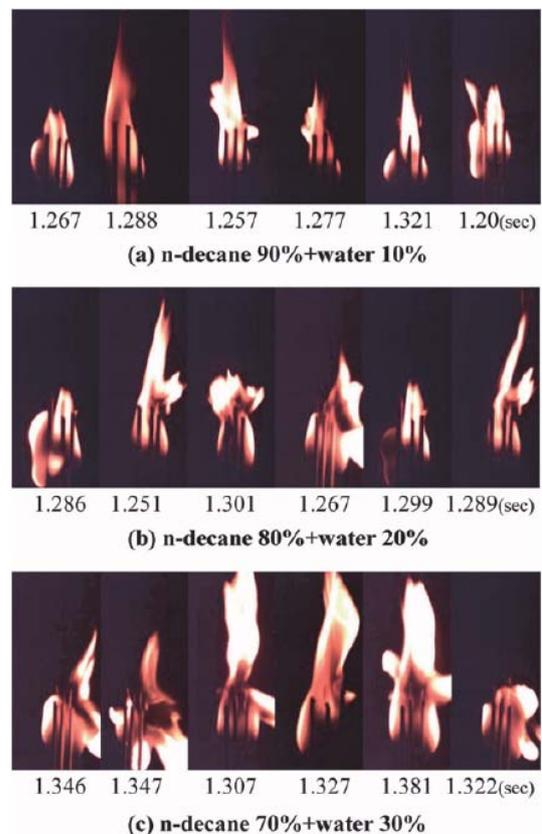
**Fig. 4.** Several cases of micro-explosion of emulsified n-decane droplet array at the starting time of micro-explosion ( $T_a=920$  K,  $D=1.0$  mm, Droplet  $n=3$ ) [18]
