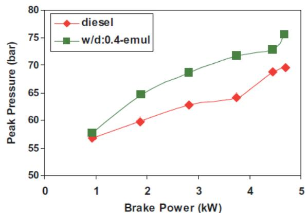
Fig. 2. Comparison of peak pressure between emulsion and diesel fuel [adapted from 15]
