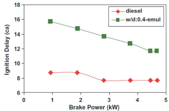
Fig. 1. Comparison of ignition delay between emulsion and diesel fuel [adapted from 15]
