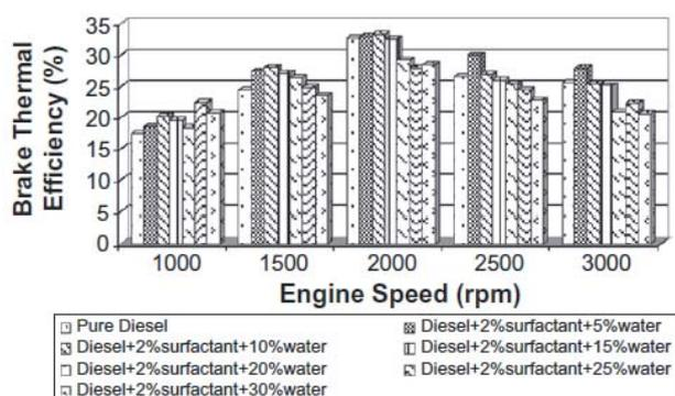
Fig. 6. Comparison of brake thermal efficiency between DWE and pure diesel [12]
