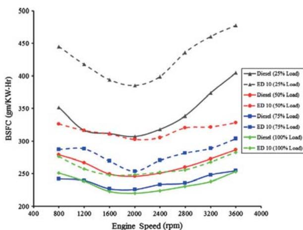
Fig. 7. BSFC for diesel and DWE10 fuels at varying engine speed and load conditions [21]
