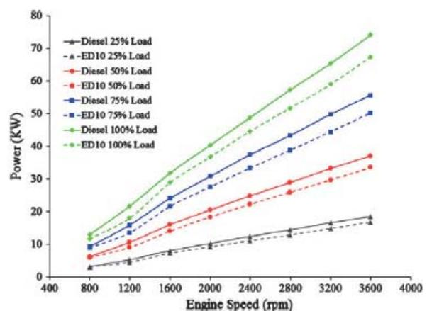
Fig. 5. Engine power output for diesel and DWE10 fuels at varying engine speed and load conditions [21]
