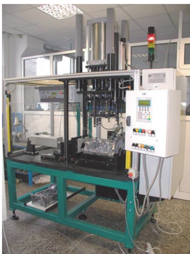
Fig. 10. Tightness control equipment for oil pan S2G- Raw.
