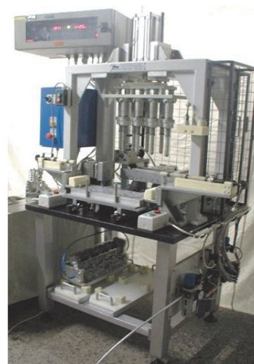
Fig. 11. Equipment for tightness control and cylinder cover marking.
