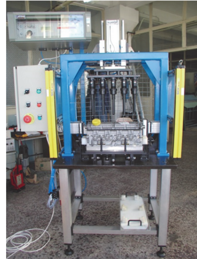
Fig. 13. Tightness control machine for assembled cylinder cover of F8Q engine.
