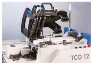
Fig. 16. The 4 over 3 with pressure bar drafting system.
