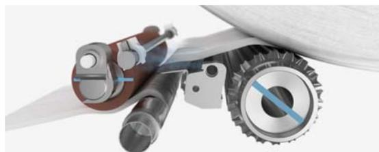
Fig. 4. Automatic lap changing and piecing system ROBOLap.
