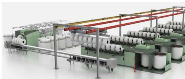
Fig. 1. Rieter E 36/E 86 combing set: one E 36 OMEGAlap and six E 86 combers
