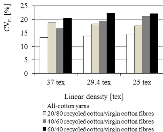
Fig. 5. CV of mass of yarns.
