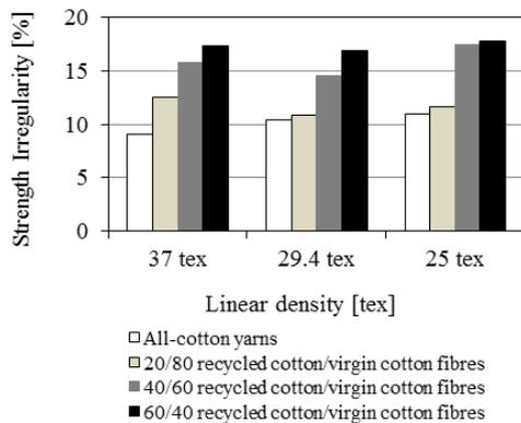
Fig. 3. Breaking strength irregularity of yarns.
