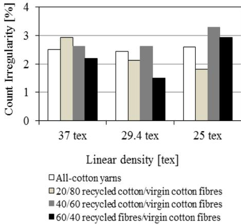
Fig. 1. Count irregularity of yarns.
