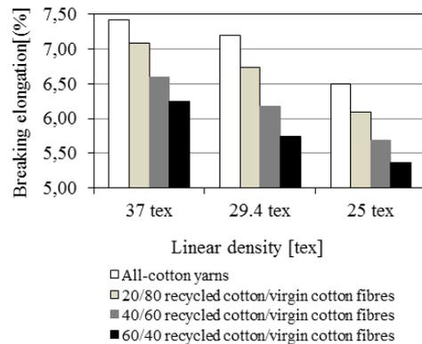
Fig. 4. Breaking elongation of yarns.
