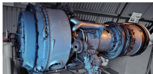
Fig. 5.2. Rolls Royce Tyne RM1C gas turbine [11].
