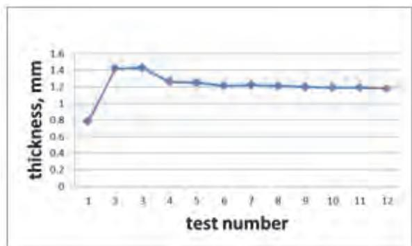
Fig. 5.b. Thickness variation of the Bc sample
