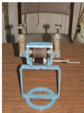
Fig. 1. Device for calibrating the thickness of the magnetic layer on textile fabrics
