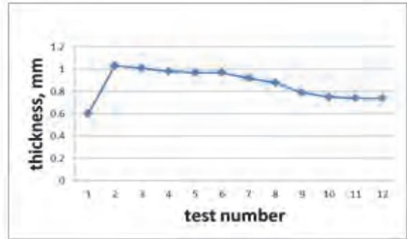
Fig. 5.a. Thickness variation of the Ac sample
