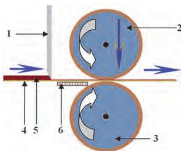
Fig. 2. Device for calibrating the thickness of the magnetic layer on textile fabrics: 1) scraper knife; 2) upper cylinder with rubber sleeve; 3) lower cylinder; 4) textile support; 5) polymeric mixture; 6) multipolar magnetic plate
