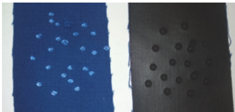
Fig. 5. Images of water drops on both sides of GoreTex material.
