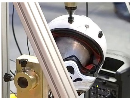
Fig. 3.5. Test de penetrare a carcasei https://www.motorcycleid.com/articles/helmet-certifications-what-are-differences-among-dot-ece-sharp-snell.html
