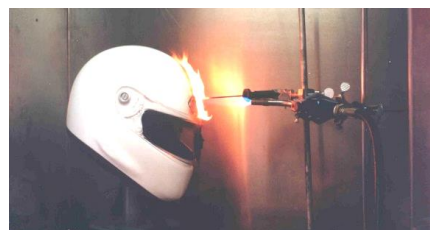
Fig. 3.7. Test de rezistență la flacără https://www.motorcycleid.com/articles/helmet-certifications-what-are-differences-among-dot-ece-sharp-snell.html
