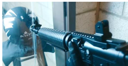
Fig. 3.6. Test de penetrare a vizierii https://www.motorcycleid.com/articles/helmet-certifications-what-are-differences-among-dot-ece-sharp-snell.html
