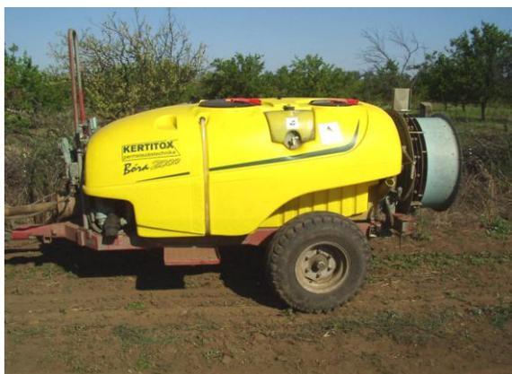
Fig. 1 KERTITOX BORA axial fan spraying machine equipped
