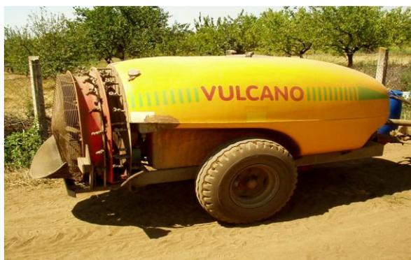
Fig. 2. VULKANO axial fan spraying machine with plant sensor
