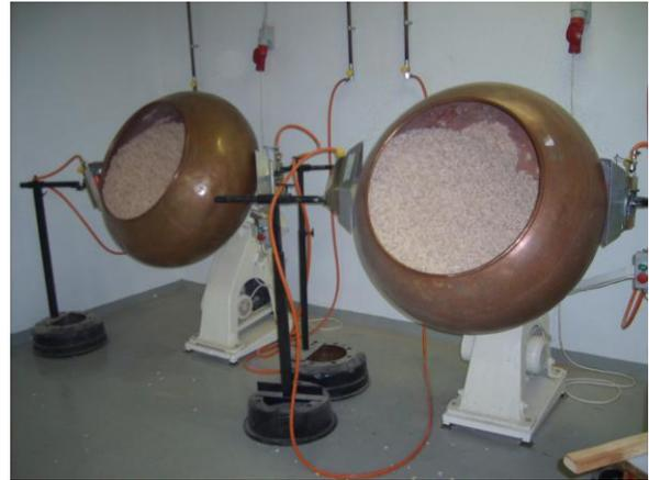
*Fig. 2* Dropping kettle
