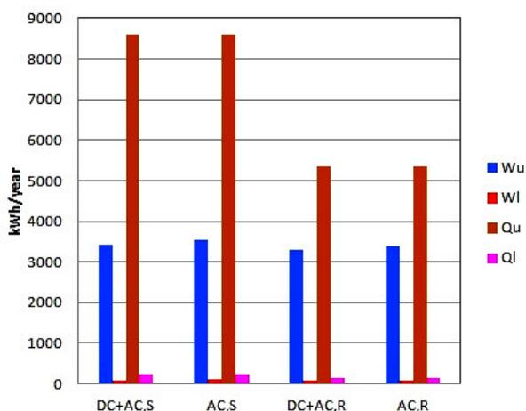
**Fig. 4.** Variation of production indicators:  $W_u$  – useful electricity of the system;  $W_l$  – loss of electricity due to interruptions;  $Q_u$  – useful heat of the system;  $Q_l$  – loss of heat due to interruptions.
