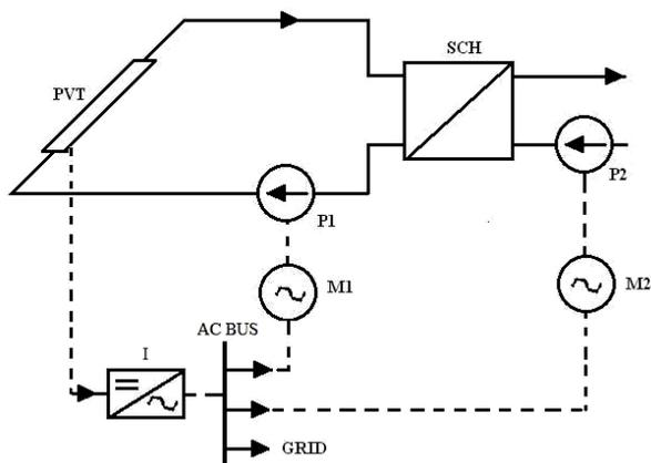
**Fig. 2.** PVT with heat exchanger and AC engine; PVT – photovoltaic-thermal panels; SCH – heat exchanger; P1, P2 – pumps; M1, M2 – AC engine; I – DC/AC inverter; AC – AC connection box
