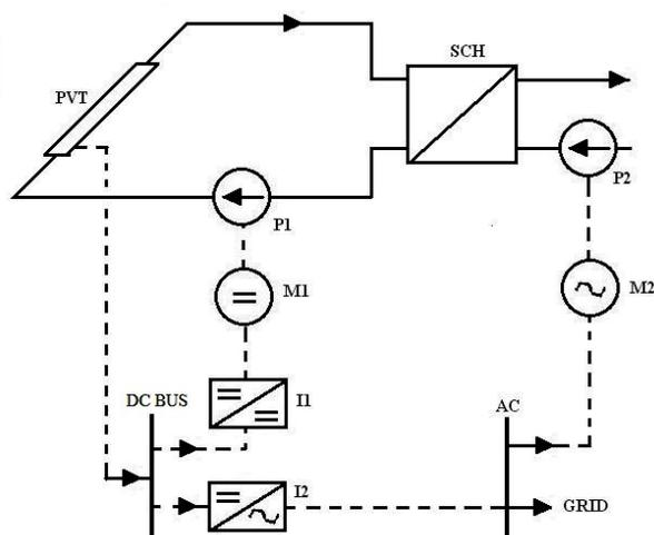
**Fig. 1.** PVT with heat exchanger and DC and AC engine; PVT – photovoltaic-thermal panels; SCH – heat exchanger; P1, P2 – pumps; M1 – DC engine M1 – AC engine; I1 – DC controller. I2 – DC/AC inverter; DC – DC connection box; AC – AC connection box.
