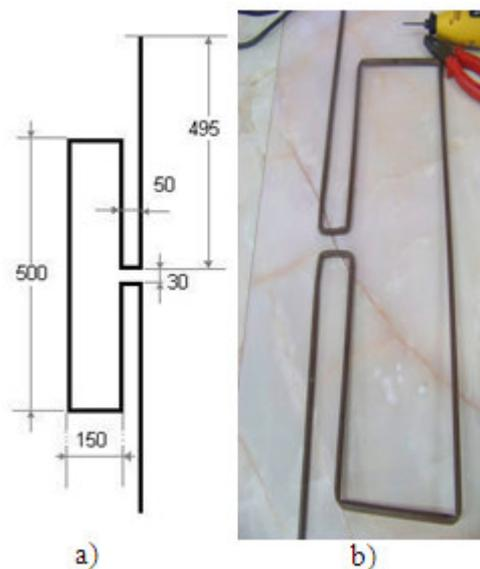
**Fig. 1** a) Elements of the antenna
