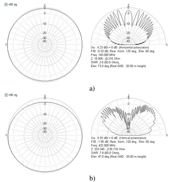
**Fig. 5** Directivity characteristic for frequency of 145 MHz
