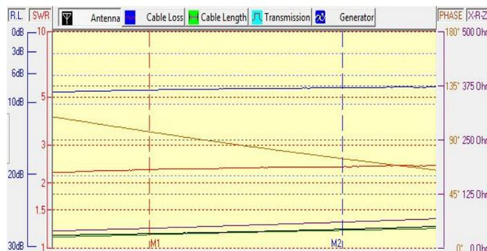
Figure 8 - Graph of evolution of antenna parameters obtained with the analyzer minivna
