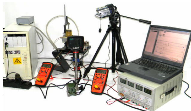
Fig.2. Experimental stand for study of transient regime of the electromechanical actuator with volatile liquid heated with Peltier elements [2]
