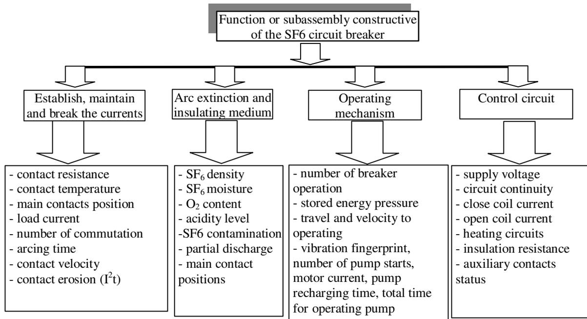
Fig.5 Monitoring parameters for an circuit breaker
