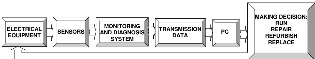
Fig. 4. Maintenance program based on condition
