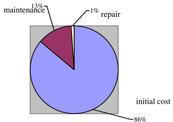
Fig. 3 Operational cost structure of an SF6 HV circuit breaker
