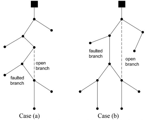
Fig. 1. Two examples of network with only one feeder. The black-filled square boxes represent the HV/MV sub-stations.
