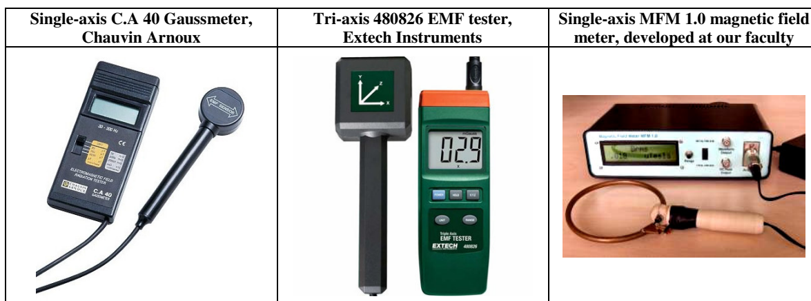
Fig. 1. Instrumentation used for the survey
