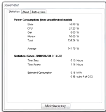
Fig. 1. Joulemeter software tool to measure the energy usage of a computer.
