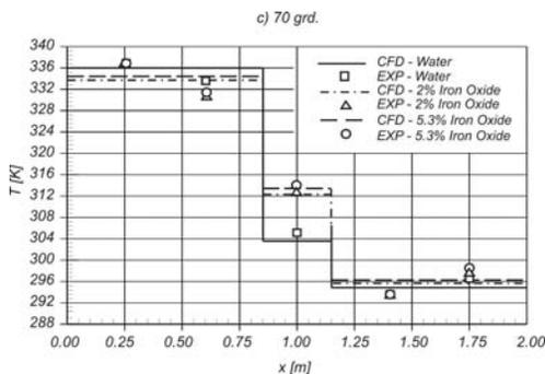
Fig. 4. Wickless heat pipe temperature distribution for different nanoparticles concentrations and an operating temperature  $T = 70^{\circ}\text{C}$ .
