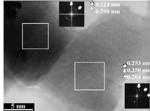
**Fig. 1.** HRTEM images, for the iron oxide sample: (a) isolated monocrystals, showing the separation interface and (b) agglomerated nanoparticles. In both images, space representations of Fourier transform are displayed.
