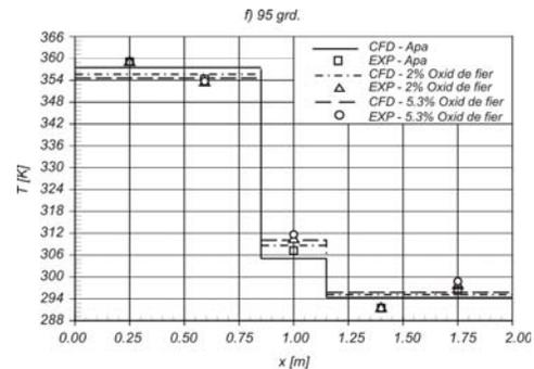
Fig. 7. Wickless heat pipe temperature distribution for different nanoparticles concentrations and an operating temperature  $T = 95^{\circ}\text{C}$ .
