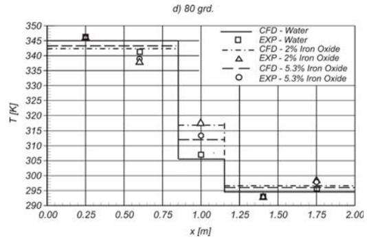
Fig. 5. Wickless heat pipe temperature distribution for different nanoparticles concentrations and an operating temperature  $T = 80^{\circ}\text{C}$ .
