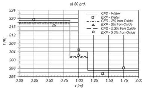
Fig. 2. Wickless heat pipe temperature distribution for different nanoparticles concentrations and an operating temperature  $T = 50^{\circ}\text{C}$ .
