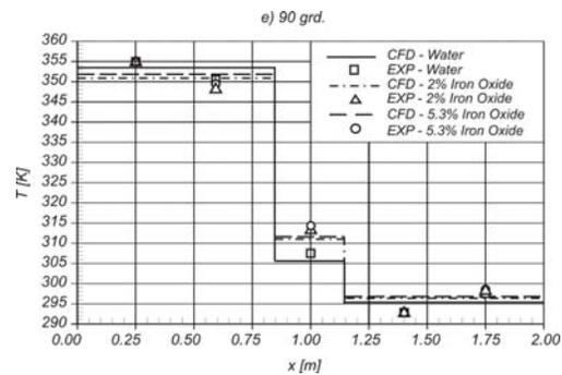
Fig. 6. Wickless heat pipe temperature distribution for different nanoparticles concentrations and an operating temperature  $T = 90^{\circ}\text{C}$ .
