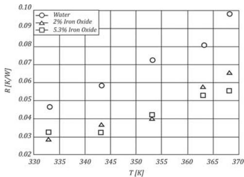
Fig. 8. Effect of iron oxide nanoparticles on total thermal resistance of the wickless heat pipe.
