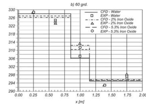
Fig. 3. Wickless heat pipe temperature distribution for different nanoparticles concentrations and an operating temperature  $T = 60^{\circ}\text{C}$ .
