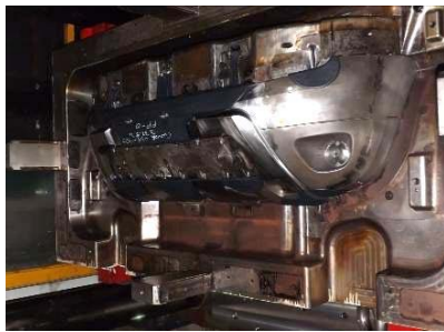
Fig. 8. Part injected at 37.69% of cylinder stroke.
