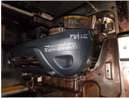
Fig 7. Part filled at 99% at commutation point.
