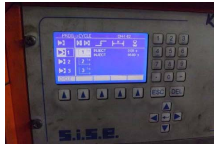
Fig 3. Full injection for each nozzle.
