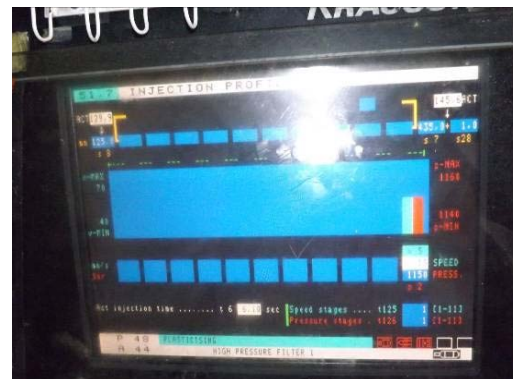
Fig. 6. Commutation point at 125 mm.
