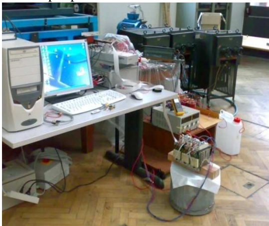
Fig. 6. Experimental setup of analyzed equipment submersed in refrigerating liquid.
