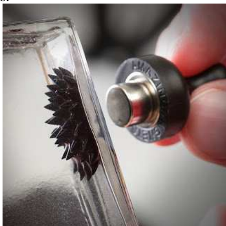
Fig. 1. Action of the external magnetic field on the ferrofluid - reproduced from [6].
