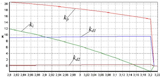
Fig. 5. The dependence of PID controller's parameters of the stability degree value.
