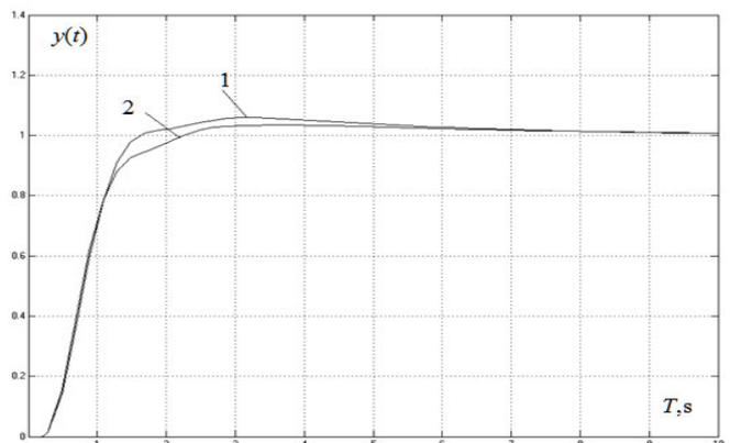
Fig. 7. The transient processes of control system with PID and PID controller.
