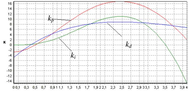
**Fig. 2.** The dependence PID controllers' parameters of the stability degree value.
