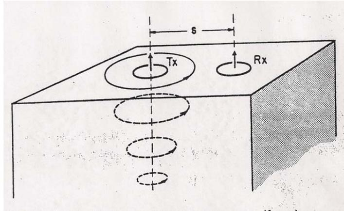
Fig. 2.1. Principle of electromagnetic soil conductivity measurement.
