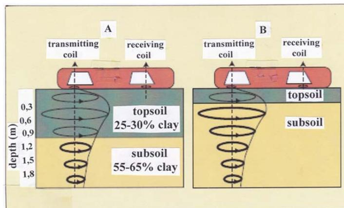
**Fig. 5.1.** The principle of operation of the device. If B is greater conductivity measured apparent that clay exhibits higher electrical conductivity.
