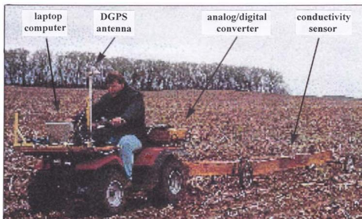
**Fig. 5.2.** Mobile equipment used for data acquisition in the field.
