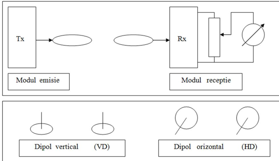
**Fig. 3.1.** Block diagram of the device and polarization types used:
