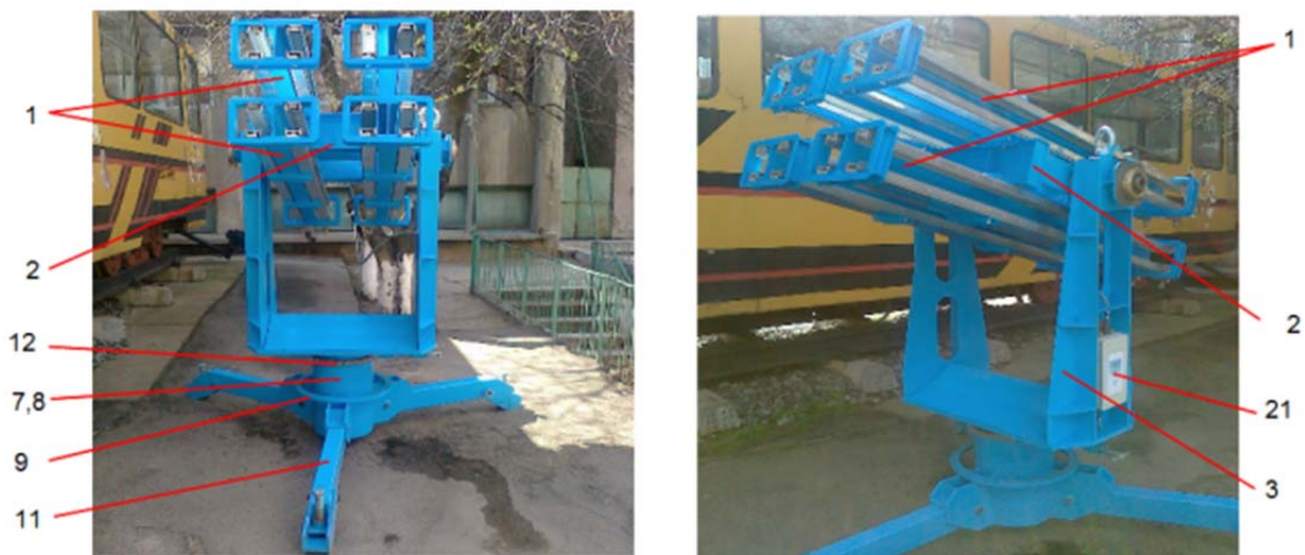
1 – Launch girder, 2 – Shelf, 3 – Azimuth/elevation cradle, 7 – Azimuth axis, 8 – Leg, 9 – Azimuth scale, 11 – Foot paw, 12 – Azimuth transducer, 21 – Distribution block
