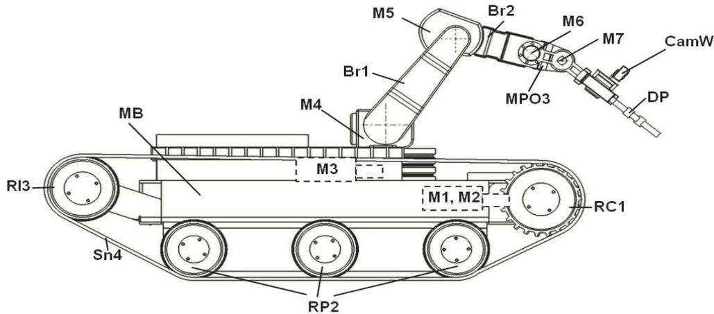
Fig. 3. The general structure of the mini-robot (side view).
