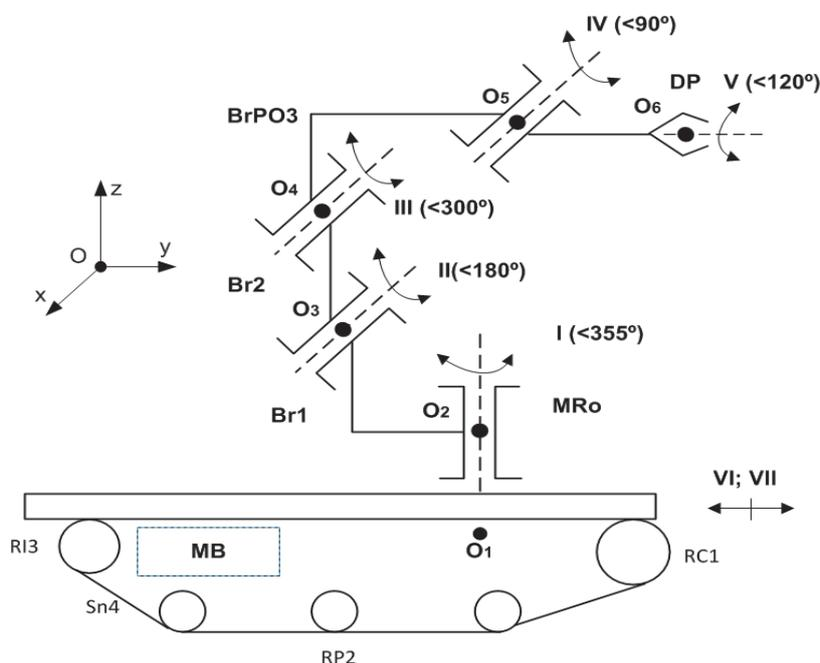
Fig. 2. The structural kinematic scheme of the mini-robot.
