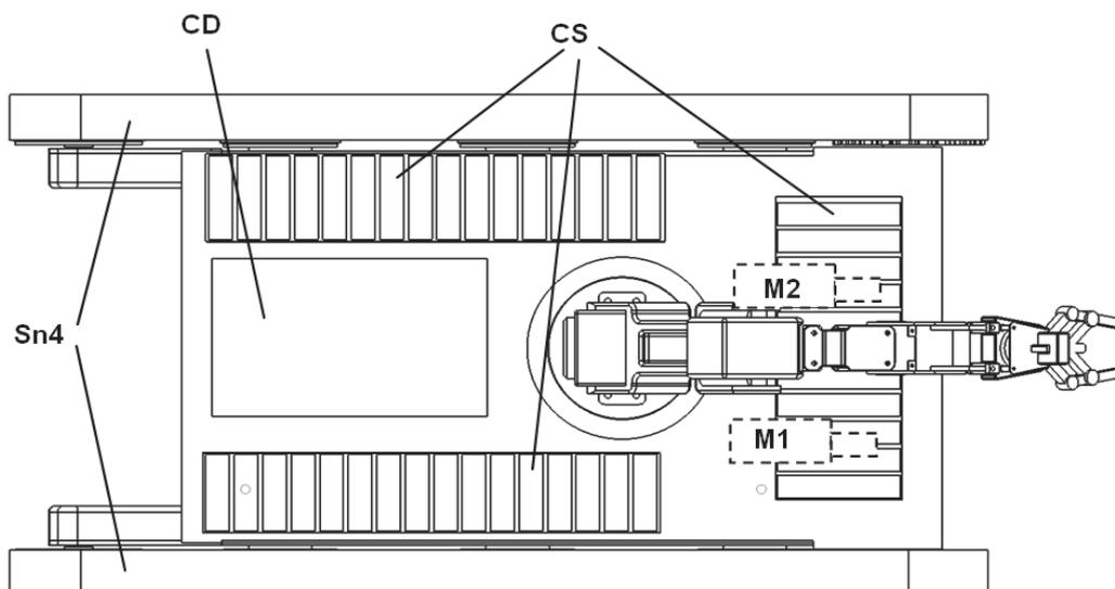
Fig. 4. The general structure of the mini-robot (top view).
