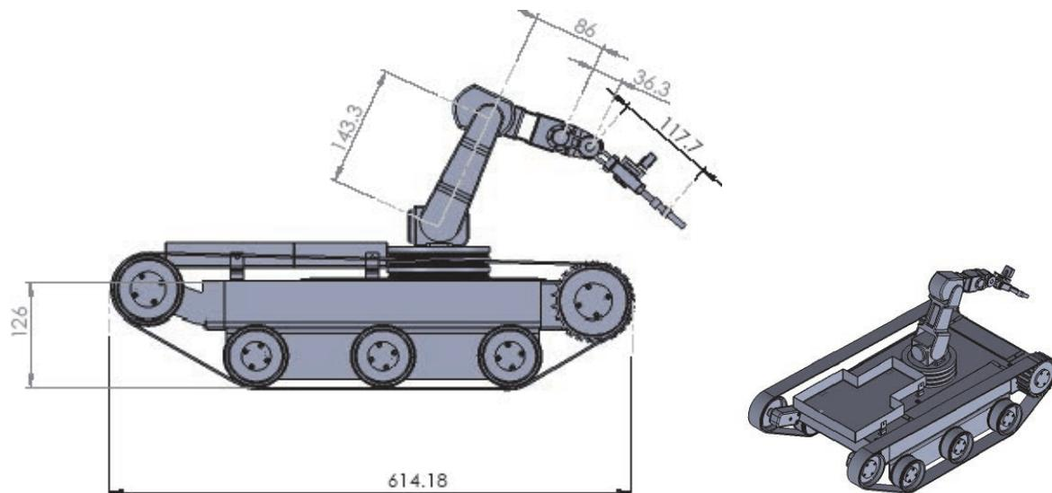
**Fig. 1.** The tracked mini-robot with electric actioning obtained from solar energy capture.
