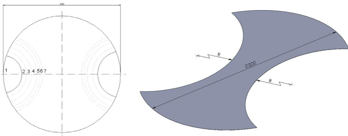
Fig. 4. The shape of the test samples used for determining the forming limit curves.
