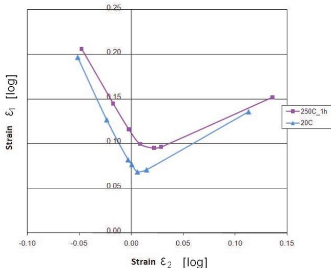
**Fig. 4.** Forming limit curves for the AZ31B alloy sheet metal in non treated and heat treated state.
