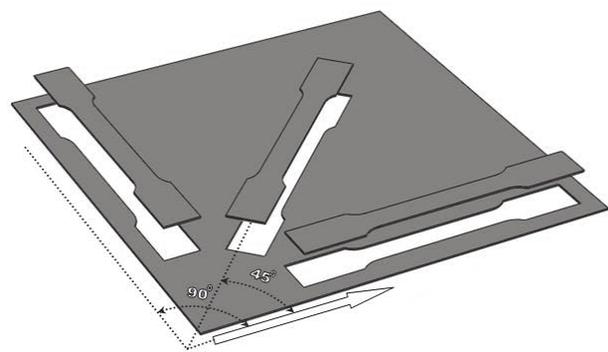
Fig. 3. Proportional test samples made at 0°, 45° and 90° to the rolling sheet direction
