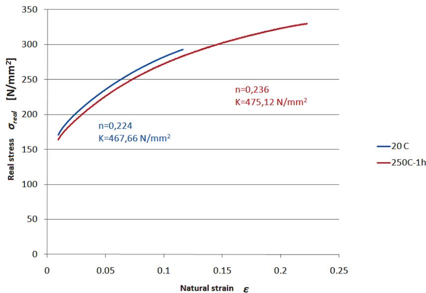
Fig. 5. Strain hardening curves for the AZ31B magnesium alloy in heat treated and non treated state.
