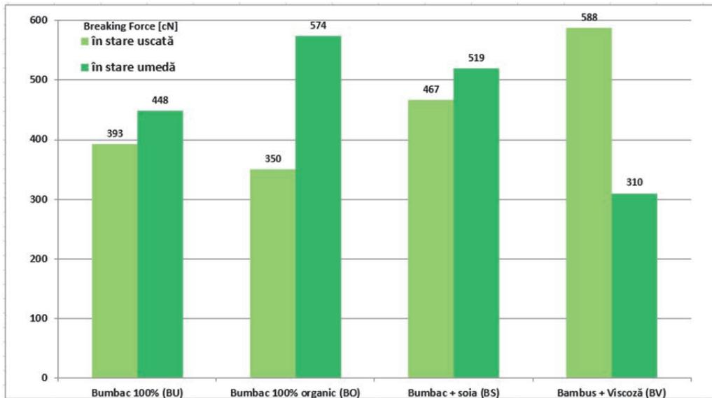
Fig. 15. The influence of moisture and raw material on the breaking force.
