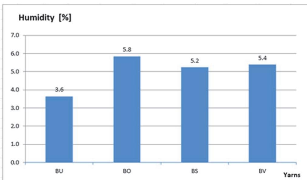
Fig. 6. The values of humidity depending on the raw material of yarn.
