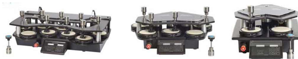
Fig. 14. Martindale Abrasion and Pilling Tester [4].
