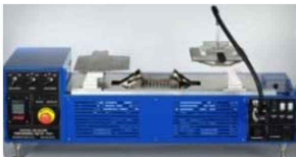
Fig. 24. Thermal Protective Performance Test Device [7].
