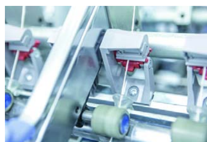
Fig. 3. USTER® SENTINEL – the ring spinning optimization system /2/.
