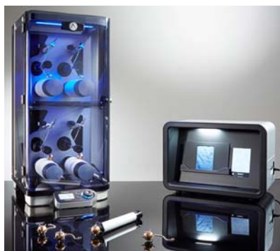
Fig. 11. ProMace, with Mace Snag Tester and the ProView Assessment Cabinet [4].
