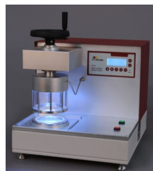
Fig. 9. Hydrostatic Head Tester [3].
