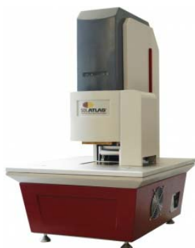
Fig. 5. FTT_Fabric Touch Tester [3].
