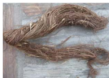
Fig. 21. Nettle fibres partially shelled by manual processes, before removing the woody stem asperities.
