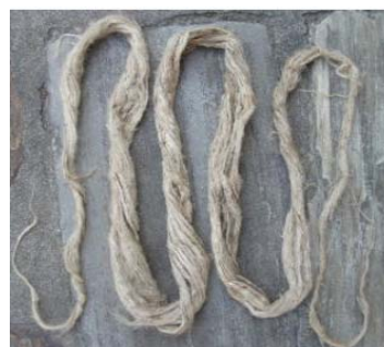
Fig. 22. Nettle fibres partially shelled by manual processes, processes after successive phases of work.
