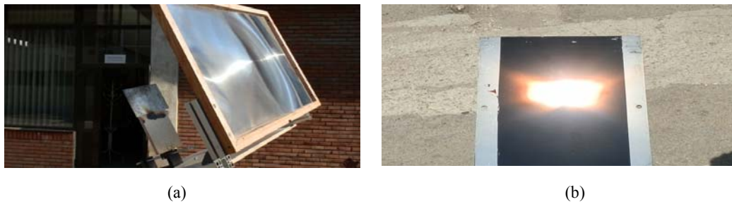
Fig. 2. Photograph of the experimental setup: (a) Fresnel lens and support plates for the focal spot; (b) the focal spot on the aluminum plate.
