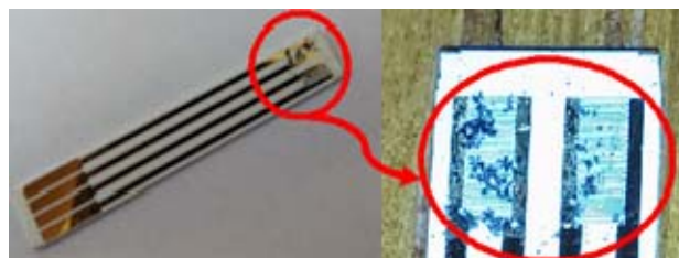
Fig. 2.1. Obtained sulfonated CNT (s-SWNT) sensor interdigitated structure.
