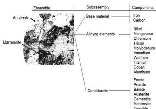
Fig. 1. The assembly of the part alloy, /7/
