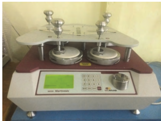
Fig. 1. Martindale Abrasion and Pilling Tester M235-SDL Atlas used for testing the abrasion resistance of upholstery woven fabrics.
