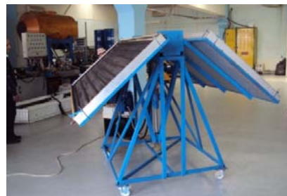
Fig. 6.2. Colector termic solar pliabil [16].
