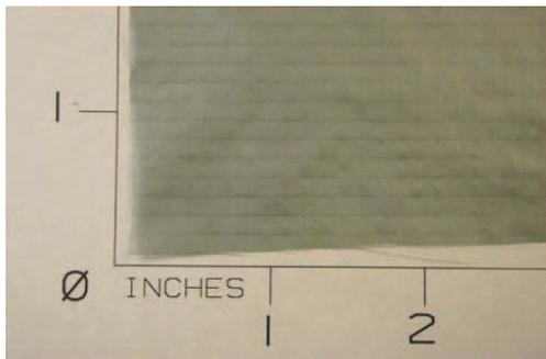
**Figure 3.** Cloth, parachute, nylon, Ty-1, Lo-Po, .5-3 cfm.
