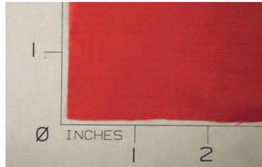
**Figure 2.** Cloth, parachute, nylon, Ty-3, 30-50 cfm.
