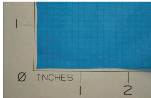
**Figure 4.** Cloth, parachute, nylon, Ty-1, zero porosity.
