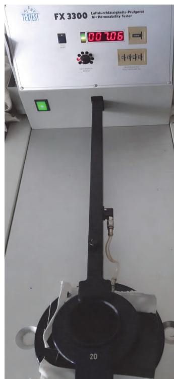
Fig. 2.1. Air permeability test – Ni sample no. 1
