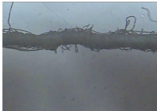
Fig. 3.2. Cotton yarn covered with a layer of copper (the yarn was extracted from the fabric)
