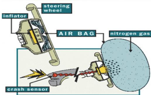
Fig. 1 Airbag module – functioning mode
