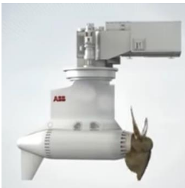
Fig. 3. Azipod systems for electric propulsion
