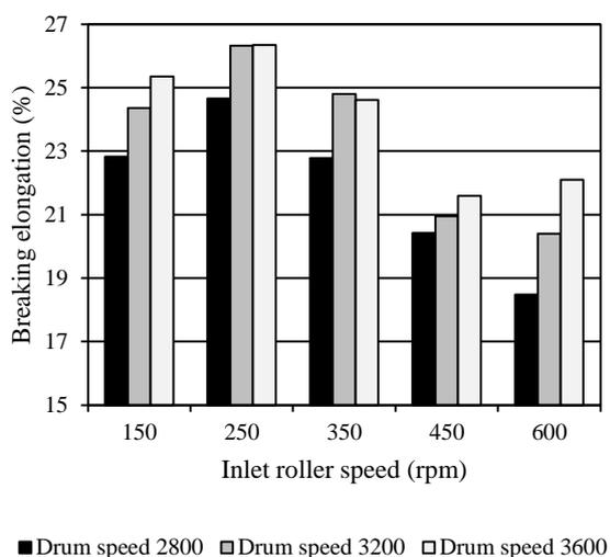
**Fig.5.** The breaking elongation of DREF-2 wool/acrylic core-spun yarns
