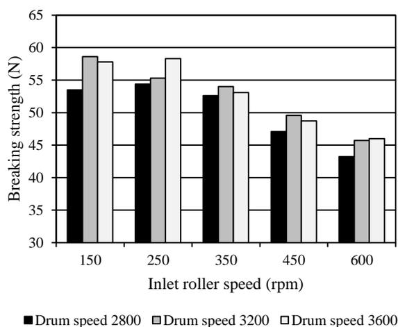
**Fig.4.** The breaking strength of DREF-2 wool/acrylic core-spun yarns
