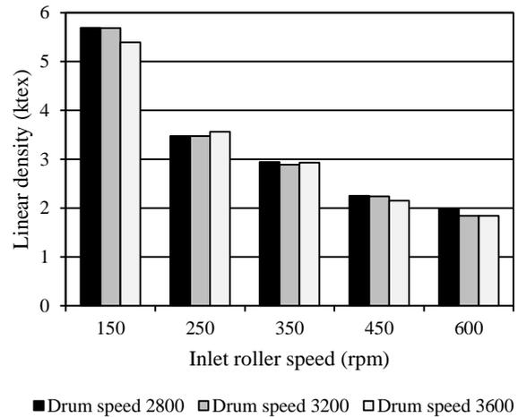
Fig.2. The linear density of DREF-2 wool/acrylic core-spun yarns
