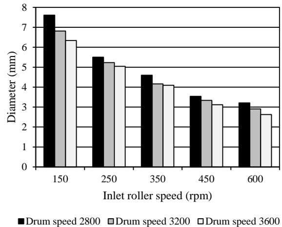
Fig.3. The diameter of DREF-2 wool/acrylic core-spun yarns
