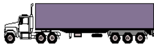
Fig. 3. Type 1 vehicle: current Single Articulated Semi-Trailer (length 19 metres, weight 42.5 tonnes Gross Vehicle Mass).
