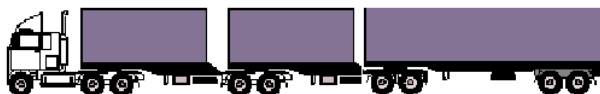
Fig. 6. Type 4 vehicle: B-Triple Tandem configuration. A PBS Vehicle (length 33 to 35 metres, weight 82.5 to 90 tonnes Gross Vehicle Mass).
