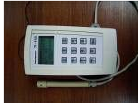
Thermoconductivity meter TK4100, \delta \leq 0,02/0.003\%
