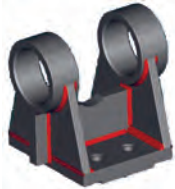
Fig. 11. Support made from welded semi-product.
