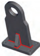
Fig. 9. Support made from welded semi-products.
