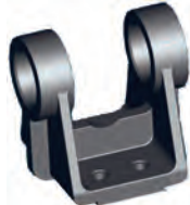
Fig. 12. Support made from cast semi-products.
