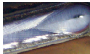
Fig. 7. The key hole, a characteristic for laser welding.
