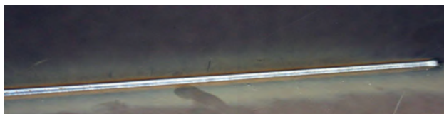
Fig. 10. Aspect of a weld joint obtained on steel 1.4541 plate using brazing with CuAl8.
