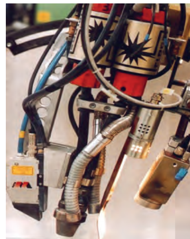
Fig. 12. Tandem® welding head with two optical sensors : a laser one for the shape (left) and a classical position detector (right).
