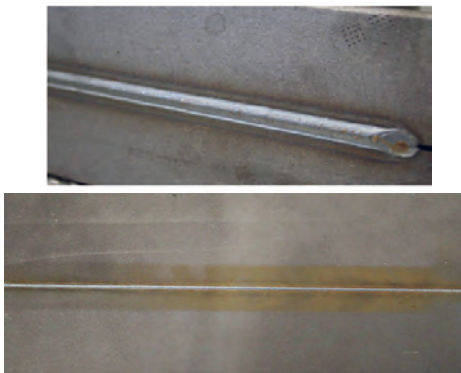
Fig. 9. Front and back side of weld joints, welded using LaserHibrid procedure on 6mm thick plates consisting of the material St 37.1; notice the extreme thin assembling of the weld groove (approx. 20°).
