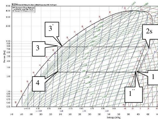
Fig. 2. Usual operating cycle, with superheating and subcooling (p-h coordinates)
