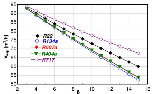
Fig. 7. Refrigerant volume rate at compressor inlet
