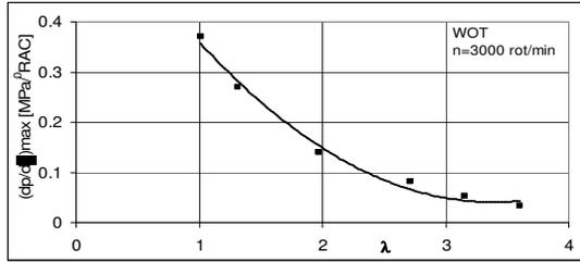
Fig. 4. Maximum pressure rate versus air fuel ratio at full load and 3000 rpm
