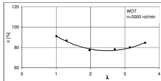
Fig. 8. Indicated specific fuel consumption versus air to fuel ratio at full load and 3000 rpm
