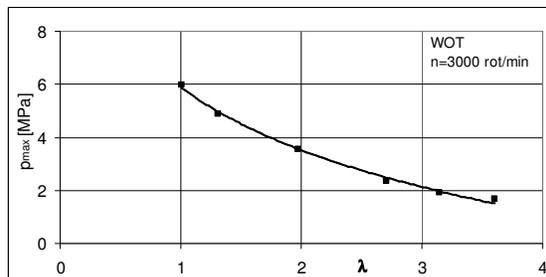
Fig. 3. Maximum pressure versus to air fuel ratio at full load and 3000 rpm
