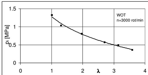
Fig. 6. Indicate mean effective pressure, IMEP, versus air to fuel ratio at full load and 3000 rpm
