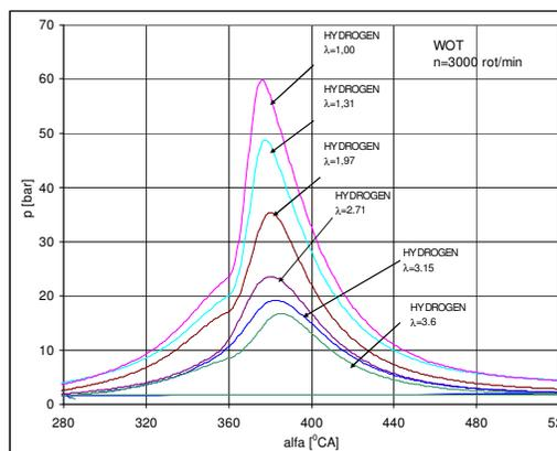
Fig. 2. Pressure diagrams at full load and 3000 rpm
