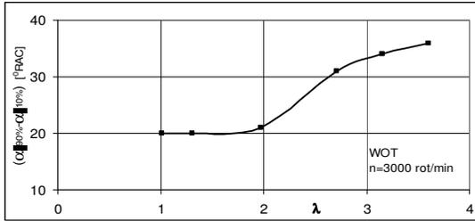
Fig. 5. Combustion time period versus air fuel ratio at full load and 3000 rpm
