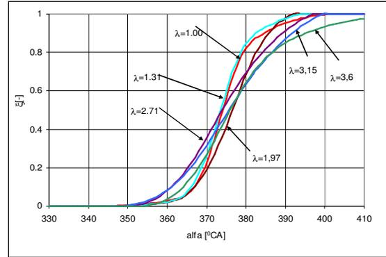
Fig. 7. Heat release versus crankshaft angle at full load and 3000 rpm
