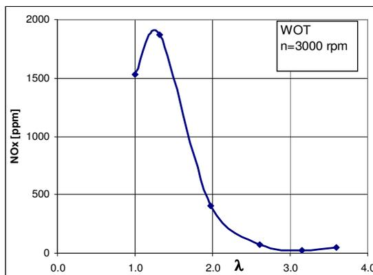
Fig. 9. Relative NO<sub>x</sub> emissions versus air to fuel ratio at full load and 3000 rpm
